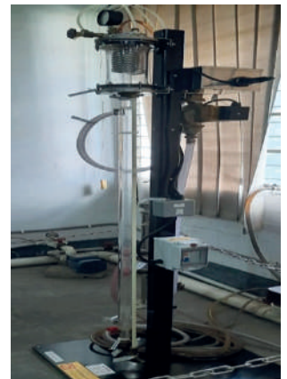
Flow boiling regime demonstration apparatus.
