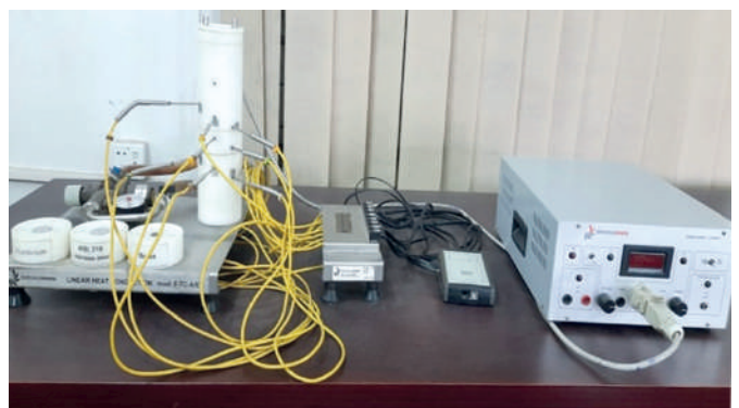
Thermal Conductivity Meter with Linear Heat Conduction Module is used to determine the thermal conductivity of metals/metal alloys.
