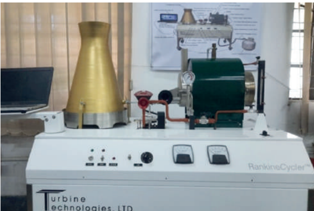
RankineCycler™ is a classroom-sized turbine power plant lab for thermodynamic steam power education.
