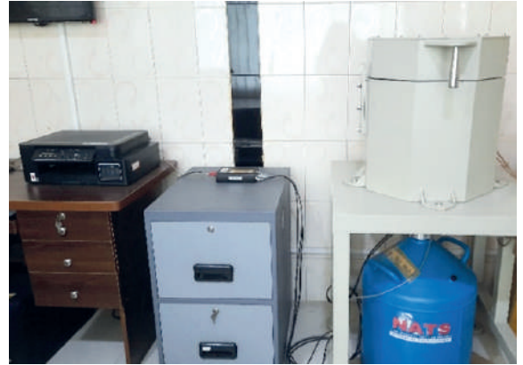
High Purity Germanium (HPGe) radiation detector
